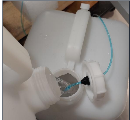
Figure 3.135 Filling the Reservoir
