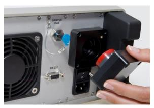
As an option, the 973-SF<sub>6</sub> is now available with integrated, industry standard chemical-based SO<sub>2</sub> measurement – another indicator of potential problems within gas-insulated equipment. The measurement cell is conveniently located on the rear panel for easy user replacement when needed (about every two years). Low cost, precalibrated, interchangeable modules make this swap-out a simple, two minute field operation.
