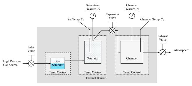
Figure 2: Schematic Diagram of the Two-Pressure Method
