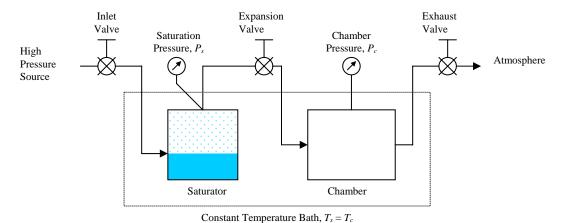
**Figure 1:** Simplified Schematic Diagram of the Two-Pressure Method where  $T_s = T_c$
