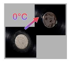
Watch the mirror closely. As soon as the mirror temperature reaches 0 °C, the ice will melt into liquid water drops (phase transition).
