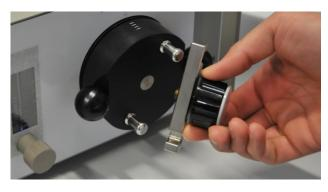
Once the clamp is removed, the black optical unit can be easily removed as shown.
