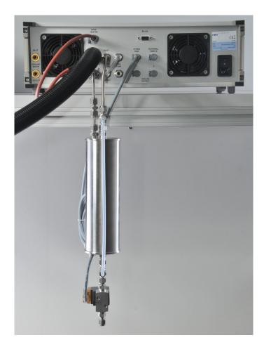
When the sample gas with a high dew point passes through the steam trap, excess water vapor condenses and is collected. The remaining gas can then pass through the 573 flow meter and sample pump without flooding. Users can also implement their own steam trap within existing installations or sampling systems. See chapter 4.4 'Back Panel' on page 23 for electrical connection of the steam trap.
