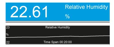
If numeric, a data line contains the value to the left, with the parameter description and unit to the right.
