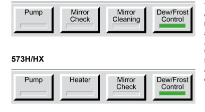
The bottom line of the display contains a row of fixed function keys. These keys are used to start and stop the *Pump*, prepare for *Mirror Cleaning* (573S only), toggle the *Heater* on/off (573H and HX only), initiate a *Mirror Check*, and switch *Dew/Frost Control* on/off.
