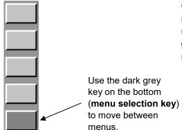
On the right hand side of the display there is a column of menu keys. The bottom, dark grey key changes the current menu by cycling to the next menu. Each of the light grey keys change their label and function based on the menu that is currently selected.
