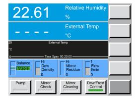
Enter the desired temperature in degrees C (21 °C in this example) and activate the **Use Fixed Ext Temp** option by touching the button. When the indicator square turns green, the fixed external temperature is active.
