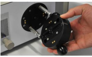
This part contains the opto-electronic components. An oval-shaped O-ring seals the measuring head. Gold contacts are located on the surface. Please avoid touching the surface of the optical unit with your fingers to avoid contamination of the contacts, the O-ring, the optical zone and the gas channel.
