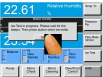
When you see the phase transition on the mirror, press the  ${\it Ok}$  button. The mirror temperature is measured at that moment and a dialog box appears with the test results.
