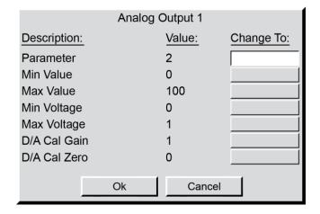
3. Then, set the scaling of the analog output signal. You want to have 0...1 VDC on the analog output to represent the 0...100 %RH. Enter *0* into the field next to the *Min Voltage* and *1* into the field next to *Max Voltage*.
