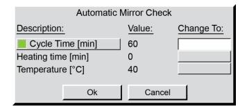
When the automatic mirror check is enabled, the *Mirror Check* key at the bottom of the screen shows a countdown timer indicating the time before the next automatic mirror check is performed. In the automatic mode, the mirror check may still be initiated manually by pressing the *Mirror Check* button.
